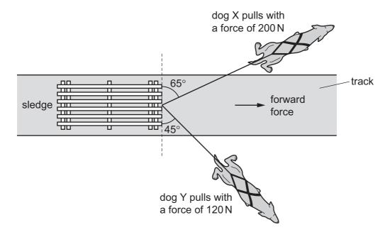
Dog X pulls with a force of 200 N at an angle of  $65^{\circ}$  to the front edge of the sledge. Dog Y pulls with a force of 120 N at an angle of  $45^{\circ}$  to the front edge of the sledge.
