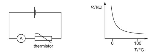
Which diagram could represent the temperature scale on the ammeter?
