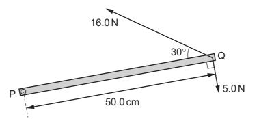
Two forces of 16.0 N and 5.0 N are in the horizontal plane and act on end Q as shown in the diagram.
